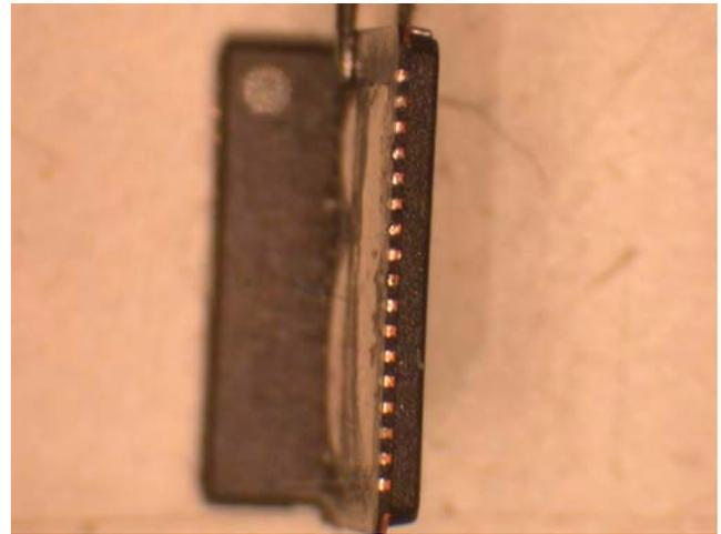
**FIGURE 17. FINISHED TINNED THERMAL LAND ON QFN**
