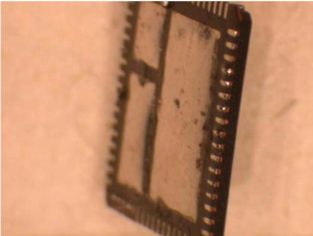
**FIGURE 16. FINISHED TINNED THERMAL LAND ON QFN**
