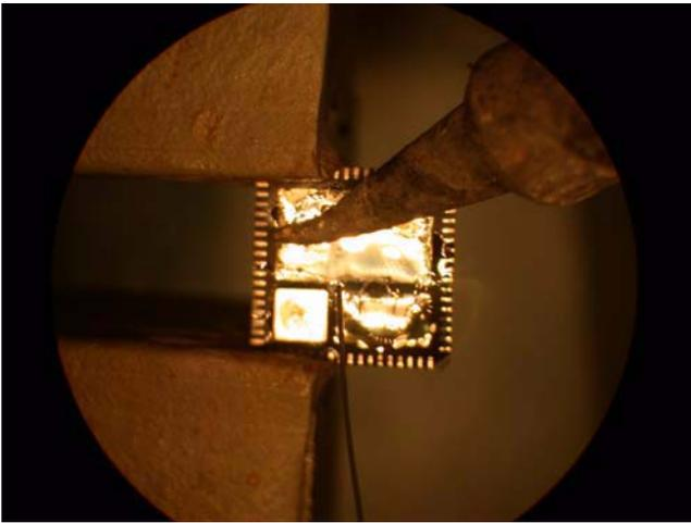
**FIGURE 15. TINNING OF THERMAL LAND ON QFN (90% COMPLETE)**
