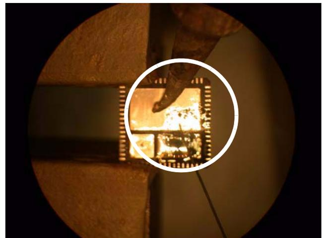
FIGURE 14. TINNING OF THERMAL LAND ON QFN (25% COMPLETE)
