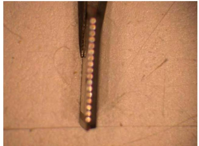
FIGURE 13. CALIPER THICKNESS MEASUREMENT OF REPLACEMENT QFN
