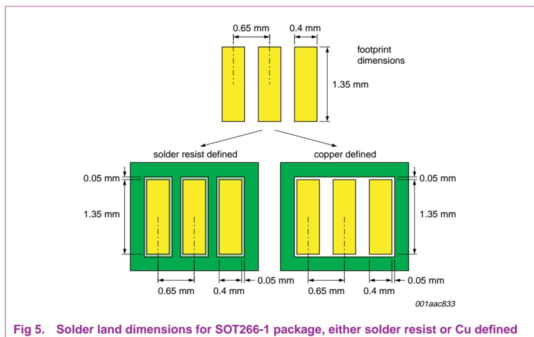
Fig 5. Solder land dimensions for SOT266-1 package, either solder resist or Cu defined
