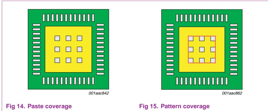
The paste printing pattern for exposed die pads is illustrated with an example, see [Figure 16](#). A HVQFN48 with an exposed pad of 5.1 mm × 5.1 mm, for example, should have nine solder paste deposits that are arranged in a three-by-three array. The solder paste deposits are 0.76 mm × 0.76 mm, and the distance between them is 0.37 mm.
