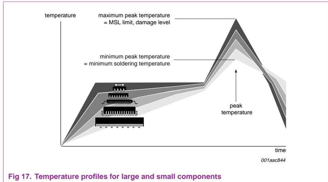
Fig 17. Temperature profiles for large and small components
