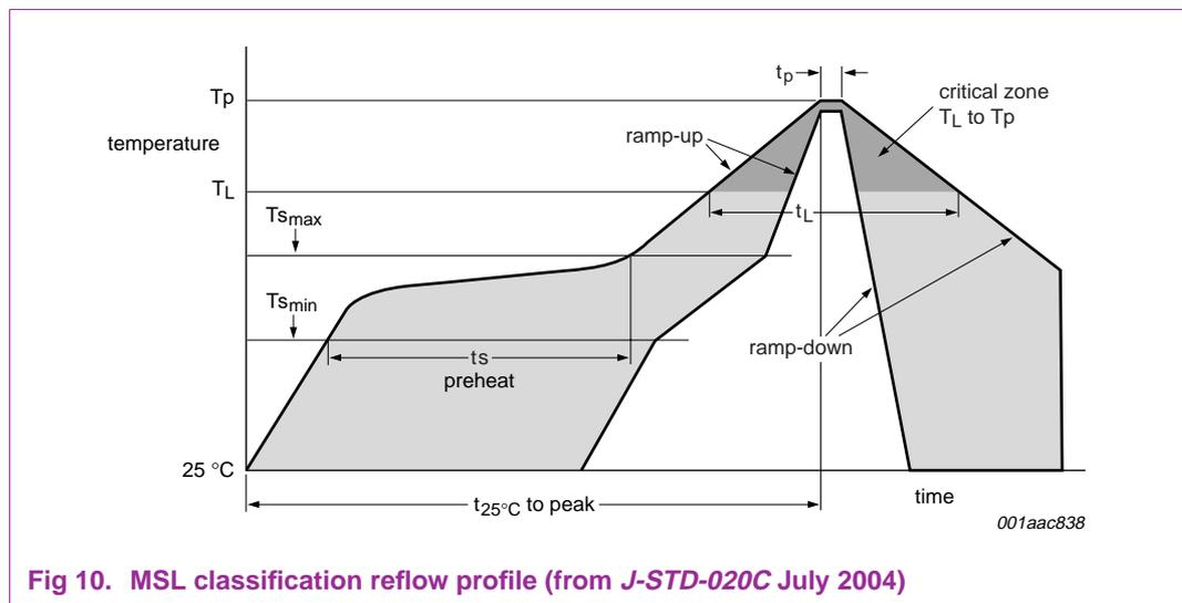
Depending on the damage after this test, an MSL of 1 (not sensitive to moisture) to 6 (very sensitive to moisture) is attached to the IC package. For every product, this MSL is given on a packing label on the shipping box. Each package is rated at two temperatures, for SnPb and Pb-free soldering conditions. An example of a packing label is given in [Figure 11](#).
