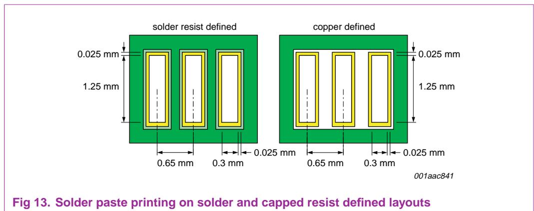
**Fig 13. Solder paste printing on solder and capped resist defined layouts**
