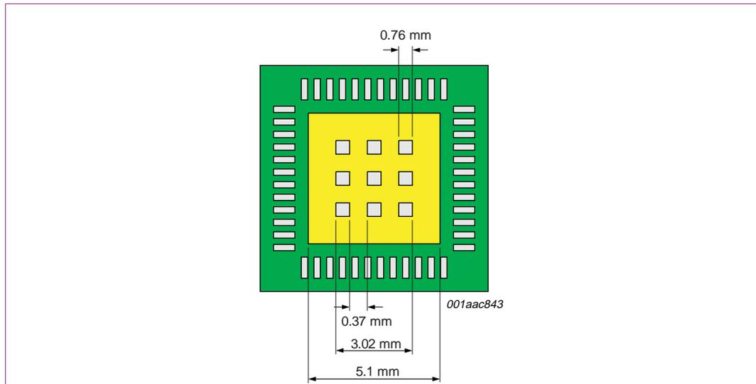
**Fig 16. Solder paste dimensions on the land area for an exposed die pad of HVQFN48**
