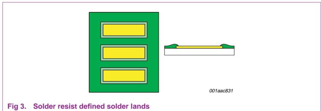
**Fig 3. Solder resist defined solder lands**
