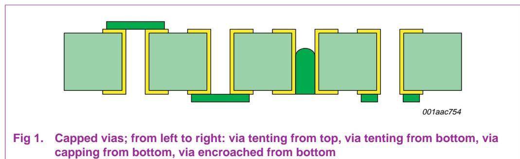
**Fig 1. Capped vias; from left to right: via tenting from top, via tenting from bottom, via capping from bottom, via encroached from bottom**
