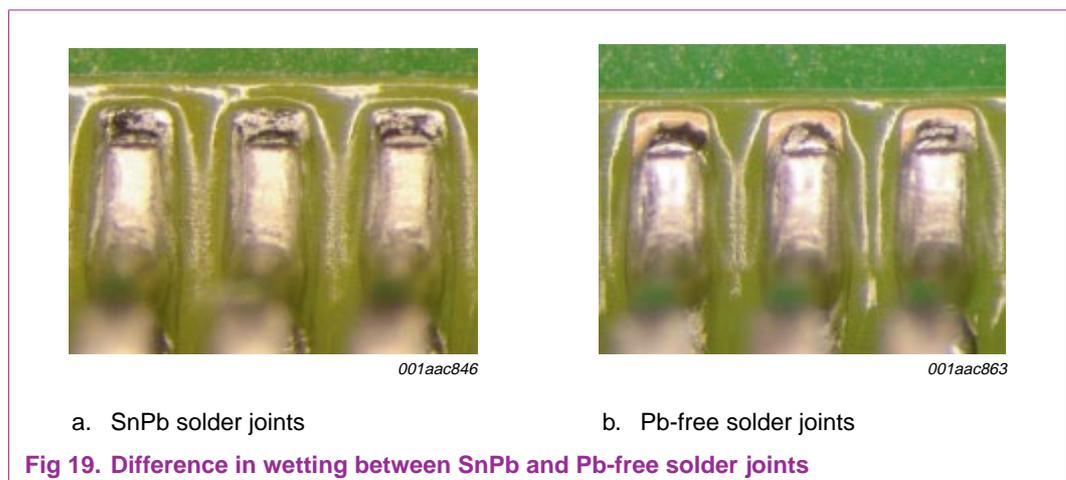
**Fig 19. Difference in wetting between SnPb and Pb-free solder joints**
