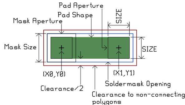
Pads and lines are represented in this way because this is how lines are specified in RS-274-X (Gerber) files which are used for creating the masks used in board manufacturing. In fact, older mask making equipment created lines in precisely this fashion. A physical aperture was used to pass light through onto a photosensitive film.
