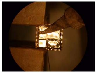
FIGURE 15. TINNING OF THERMAL LAND ON QFN (90% COMPLETE)
