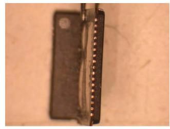
FIGURE 17. FINISHED TINNED THERMAL LAND ON QFN
