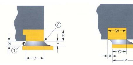
FIGURE 4. QFN TERMINATIONS
