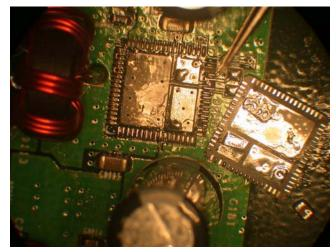
FIGURE 10. COMPONENT LIFTED OFF/REMOVED
