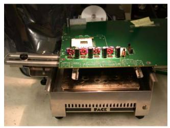
FIGURE 5. HOT PLATE REWORK STATION
