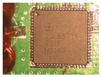
FIGURE 20. FINISHED QFN COMPONENT REPLACEMENT
