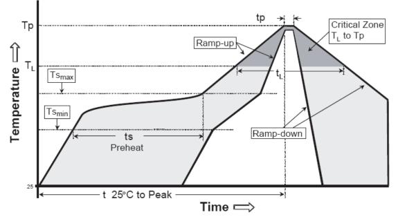
FIGURE 3. TYPICAL REFLOW PROFILE
