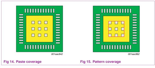
The paste printing pattern for exposed die pads is illustrated with an example, see <u>Figure 16</u>. A HVQFN48 with an exposed pad of 5.1 mm  $\times$  5.1 mm, for example, should have nine solder paste deposits that are arranged in a three-by-three array. The solder paste deposits are 0.76 mm  $\times$  0.76 mm, and the distance between them is 0.37 mm.
