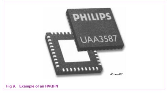
IC packages may have heat sinks at the top or the bottom of the package. A few extra remarks are made on IC packages with heat sinks at the bottom (such as HVQFNs):
